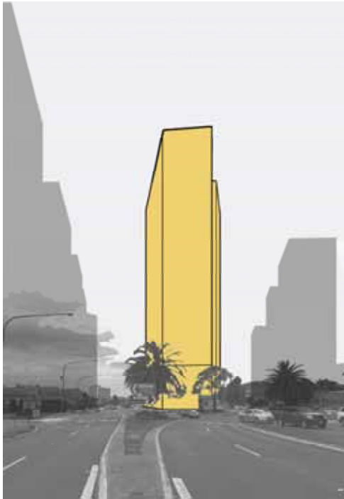
11_Slider A • 10:1 FSR • 700m2 floor plates • single loaded corridor
